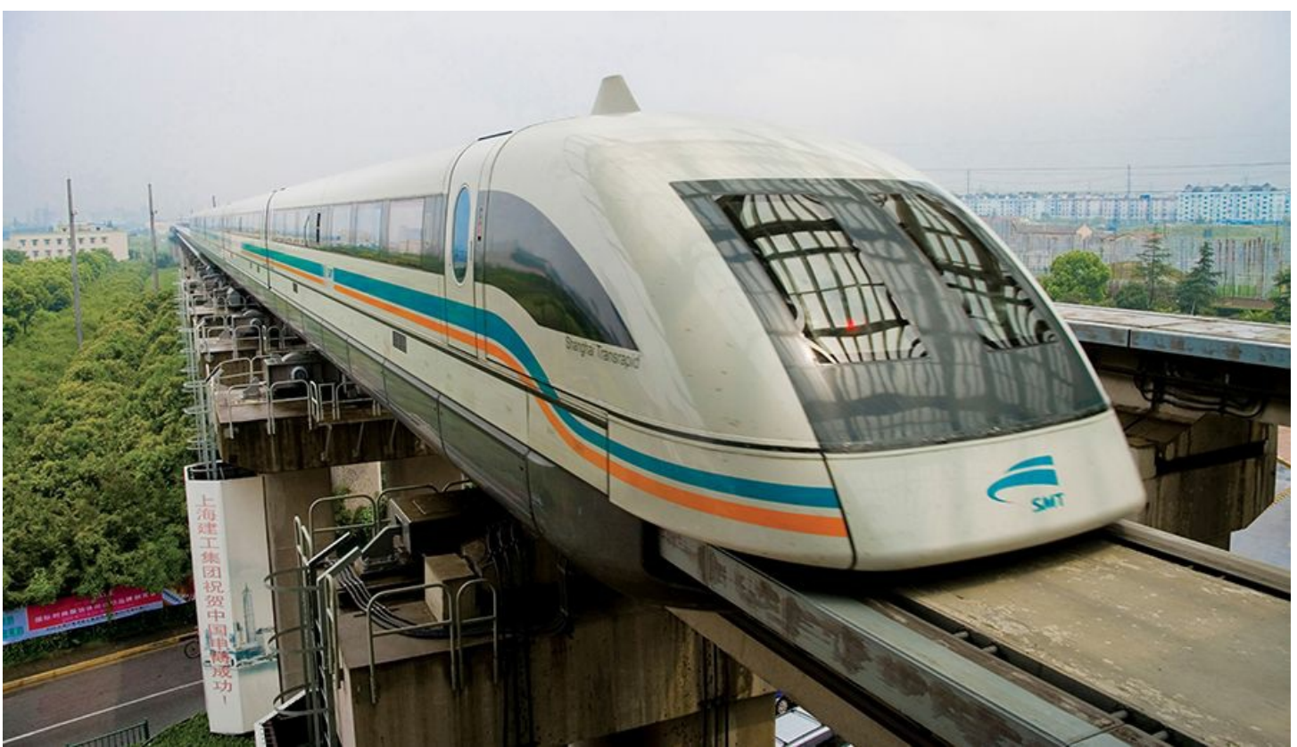
Fig. 2.7. The world's first commercial magnetically levitated train, in Shanghai, China.
